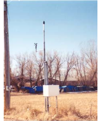
Remote Monitoring Terminal (RMT) with a weather collecting station.
