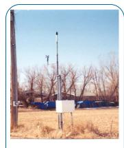
Remote Monitoring Terminal (RMT) with a weather collecting station.
