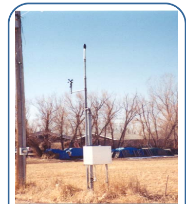
Remote Monitoring Terminal (RMT) with a weather collecting station.
